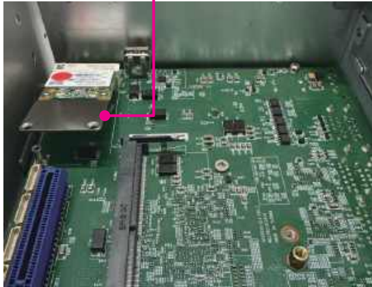
Mini-PCIe card (half-size) secured on the bracket
