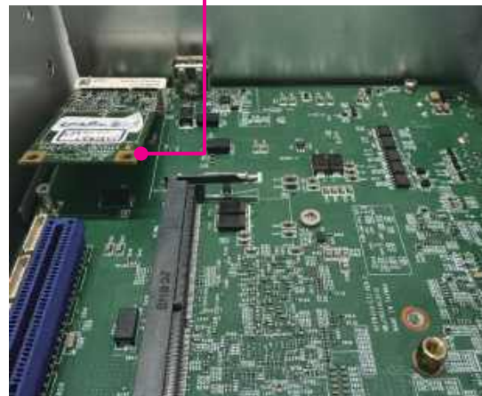
Mini-PCle card (full-size) secured on the bracket
